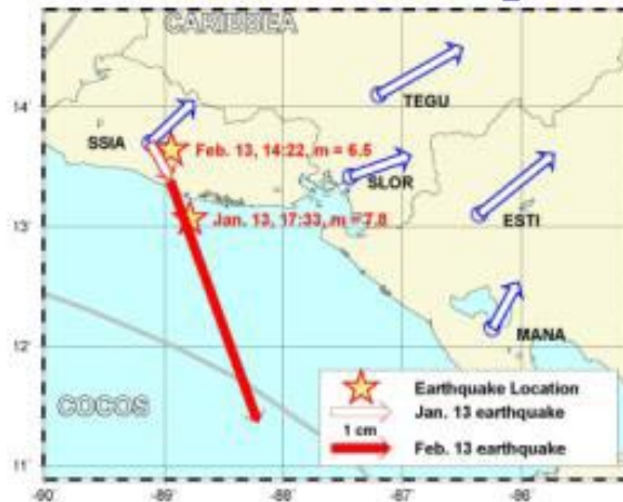
Displacements of station SSIA
