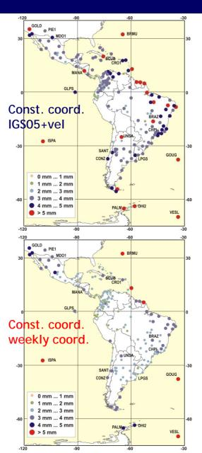
Network deformation: 3D residuals after comparing solutions aligned to the IGS05 with the primary loosely constrained solutions
