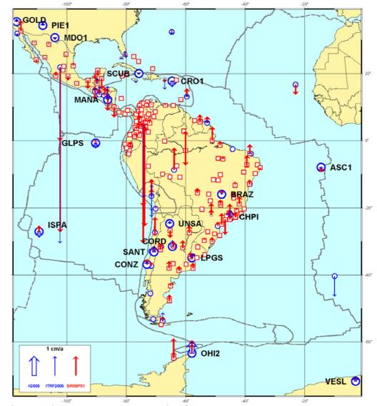
Agreement with IGS05 in position: horizontal. ~ 2.0 mm , vertical: ~ 3.5 mm in velocity: horizontal: ~ 0.5 mm/a, vertical: ~1.0 mm/a
