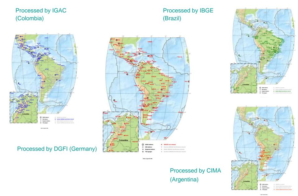
Figure 1: The four SIRGAS sub-networks of the SIRGAS-CON network
