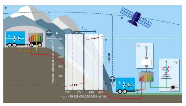
Excellent agreement between height differences from clock and from conventional geodesy: 0.19 m, but clock accuracy still two orders of magnitude below geodesy
