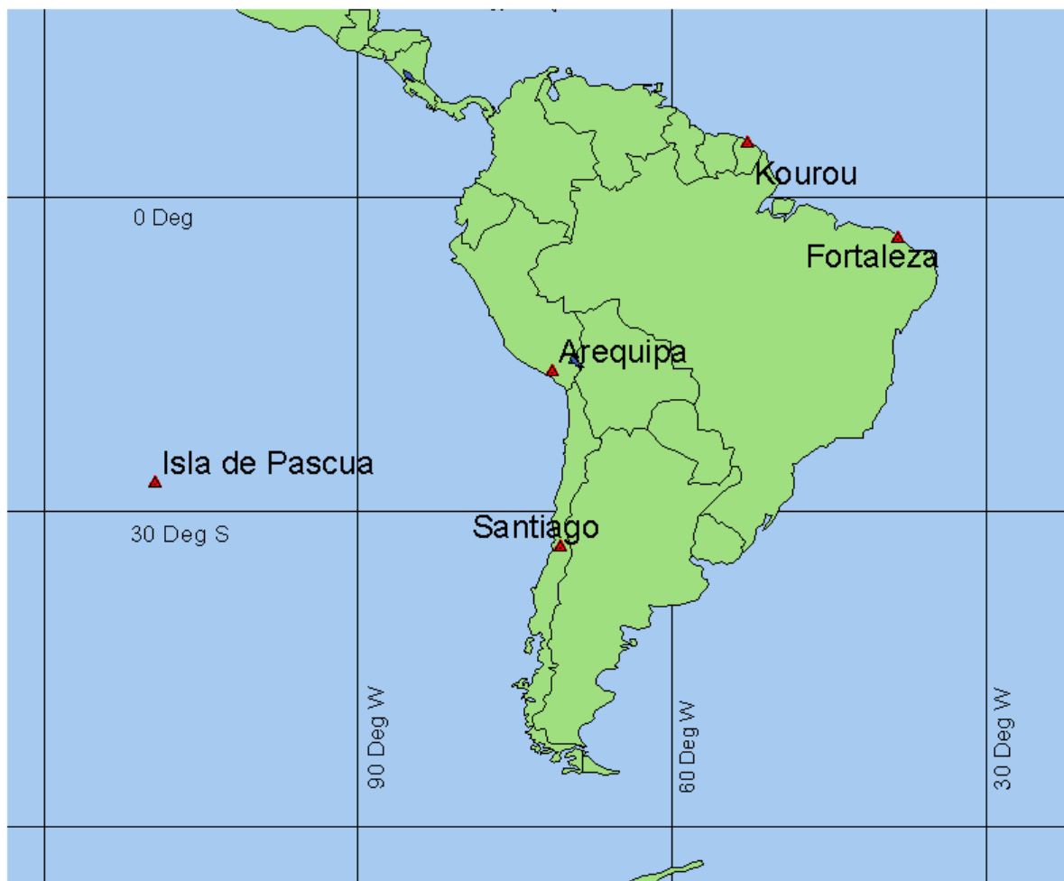
FIGURE 2.6: Geographic distribution of the IGS stations used to derive the transformation parameters from ITRF93 to ITRF94
